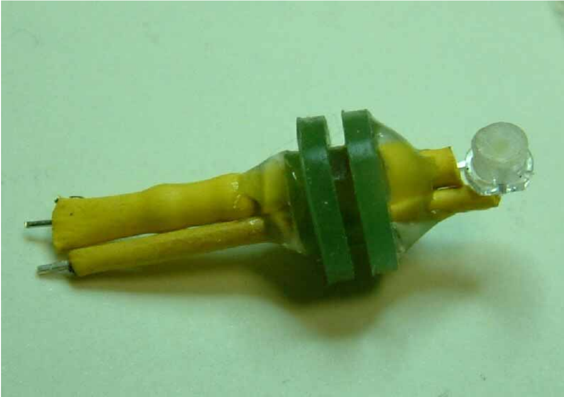
Picture 8: Complete LED assembly ready for installation
