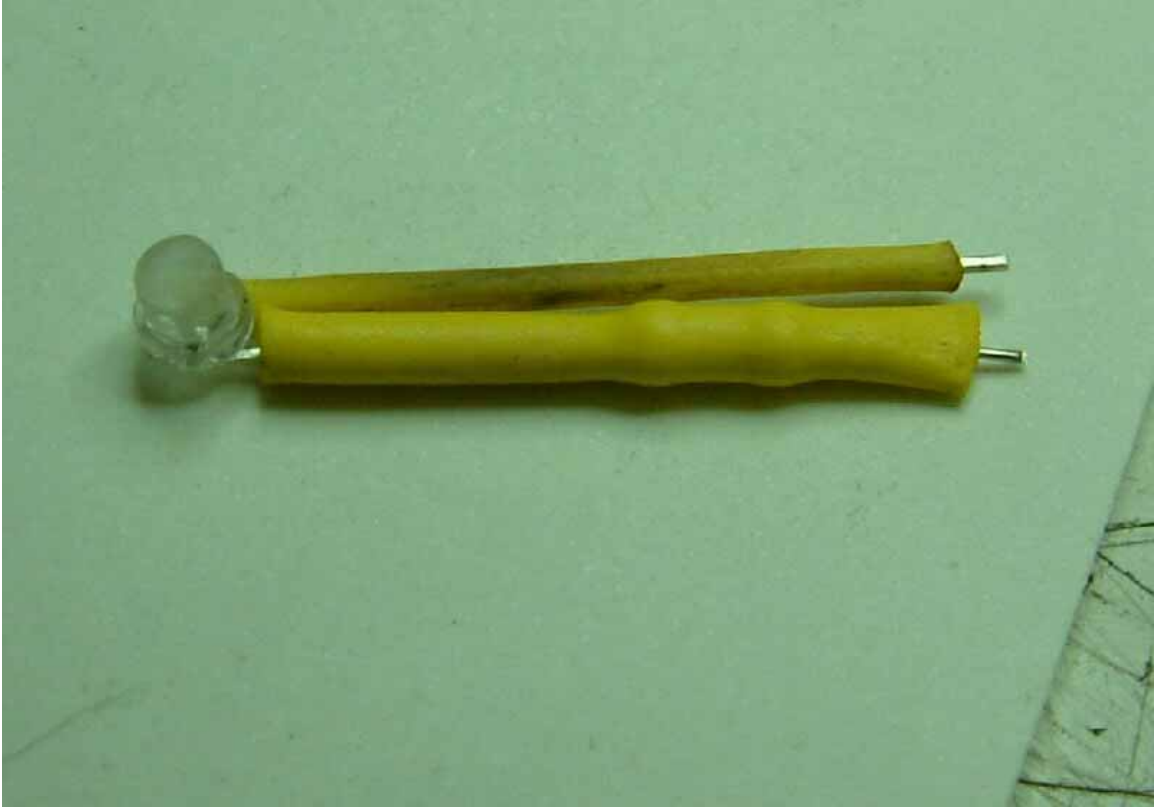
Picture 7: After the resistor is installed, cover both leads with heat shrink tubing and trim the leads to be the same length.
